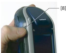
To wake up the receiver, hold the same button pressed until the screen wakes up. This will instantly restore the use context in which the receiver was before entering the Suspend mode.
