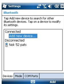
On the receiver, the name of the cell phone now appears in the list of "Disconnected" devices (meaning it is now paired with your receiver and available for a connection, but not involved yet in any connection).
